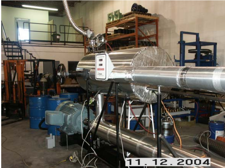
View of Test Bench Showing the Motor, Flow Meter, Choke, Reservoir and Discharge pressure gauge
